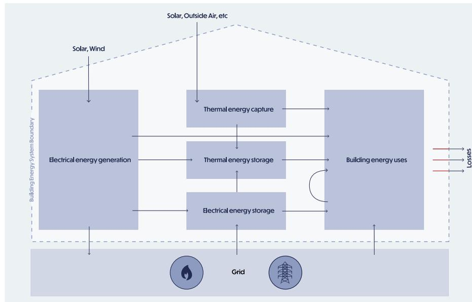
Figure 3. Considerations inside and outside the building energy system boundary
